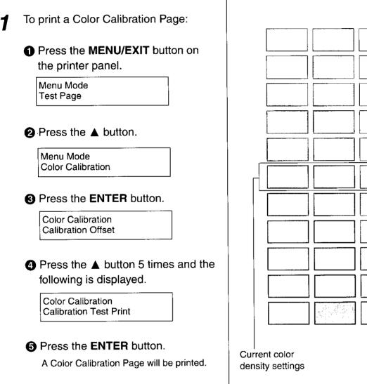
The current density setting for each color is indicated by the line enclosure on the Color Calibration Page as shown in the following example. The factory default setting for each color is 0.
