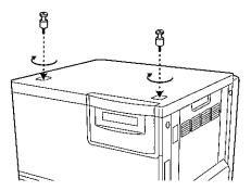
**3** Match the guide pins to the holes under the scanner, and place the scanner gently onto the printer.
