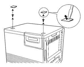
**2** Install the guide pins and tighten them with a flat-blade screwdriver.
