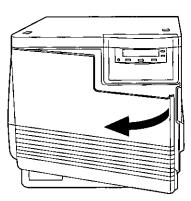
2 Turn the upper green lever clockwise until it stops and the arrows are aligned. (This tightens the internal belts to ready the unit for printing.)
