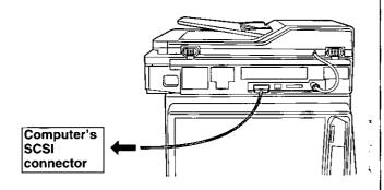
**3** Connect the SCSI cable provided to the printer's SCSI connector and to the scanner's SCSI connector.
